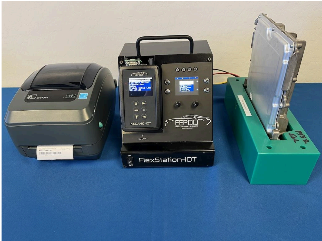
EEPod FlexStation-IOT with Label Printer and ECU POGO Pod Attachments (total cost ~$5K, depending on ECU pod type)
