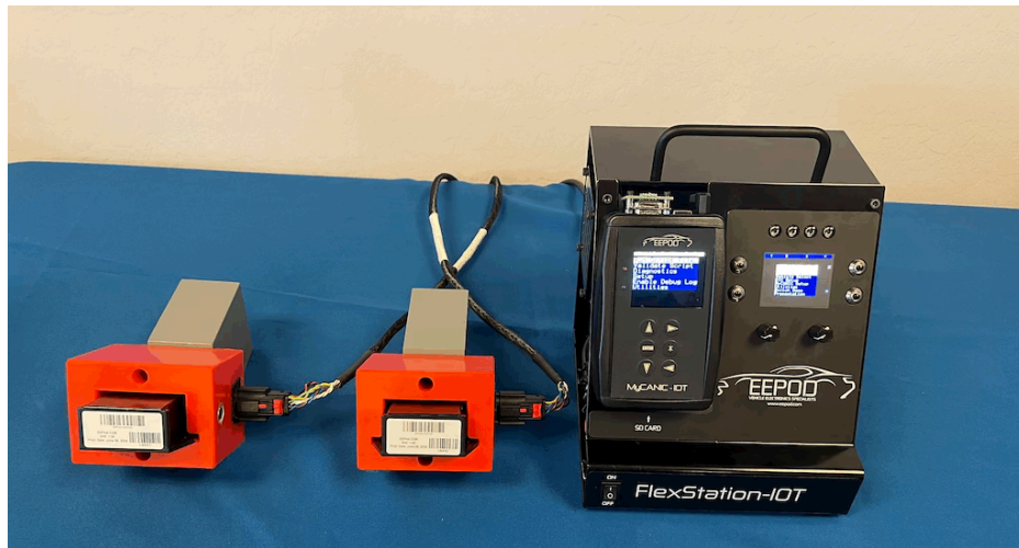
FlexStation-IOT Connected to ECUs with High Volume Pogo Pin Fixtures
